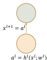
$$\frac{\partial \mathcal{L}}{\partial a^{l}} = \left(\frac{\partial a^{l+1}}{\partial a^{l}}\right)^{T} \cdot \frac{\partial \mathcal{L}}{\partial a^{l+1}}$$
